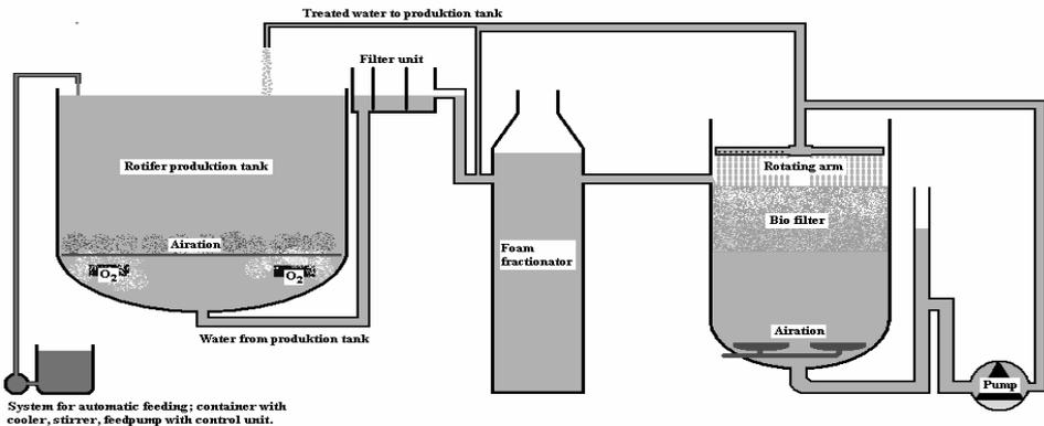
Fig. 1. Schematic view of the recirculation system.
