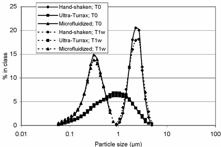
Fig. 1. Particle size distribution (at T0 and after 1 week cold storage) of ICES 30/0.6/C emulsion prepared through hand-shaking, high-shear blending (Ultra-Turrax), or microfluidization.
