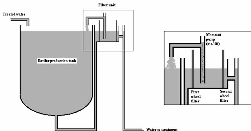
Fig. 2. Schematic view of the external filter unit.
